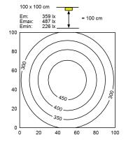
Light sourceLEDWork equipmentWithoutConnected load22 - 26 V; DCPower consumptionca. 16 W
